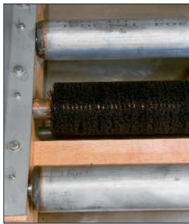
Rotary Bottom Scrubber
